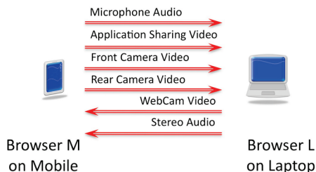
Figure 1.9 Multiple Media Streams in a Point-to-Point WebRTC Session
